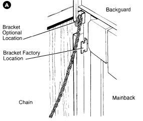
2. Fasten one end of the stability chain to the floor or wall with the long screw and washer supplied. See Fig. B. Make certain the screw is going into the wall plate at
